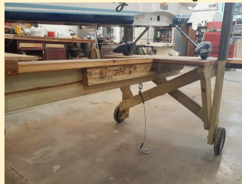
Cable attaches to a screw anchor in the ground.
