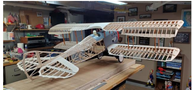
Flat gray primer on sheeting. Cowling covers and blisters to be added.
