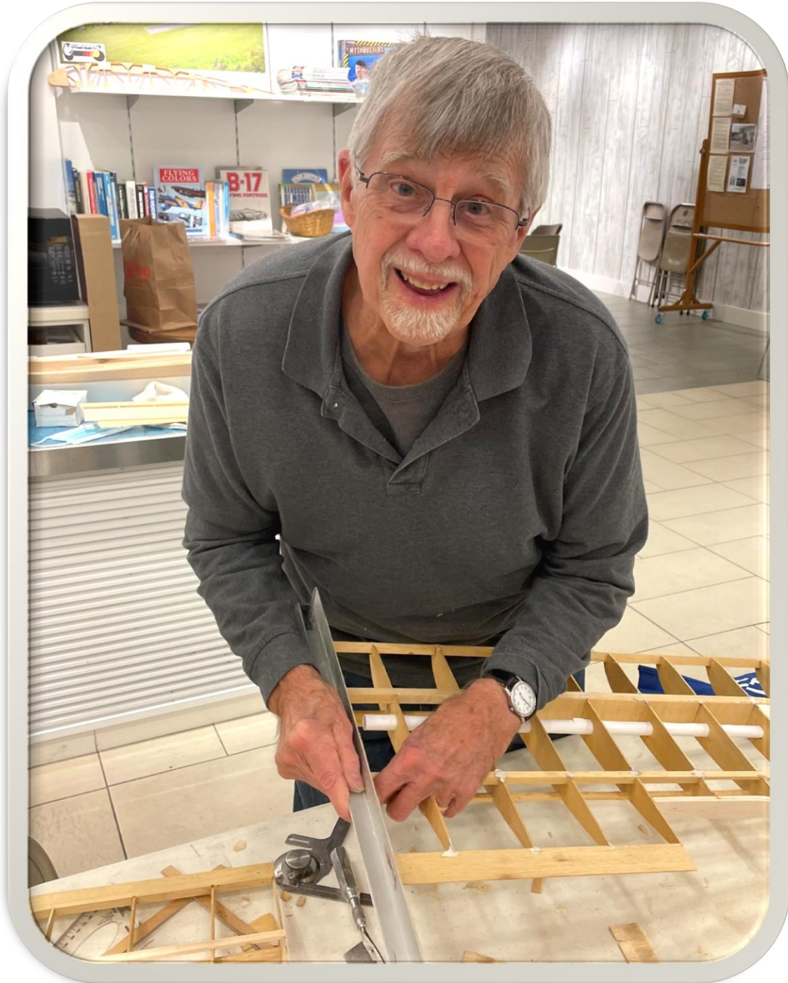
Greg R, continues work to add ailerons to the Wing of Electrified Sig Kadet Senior Kit
