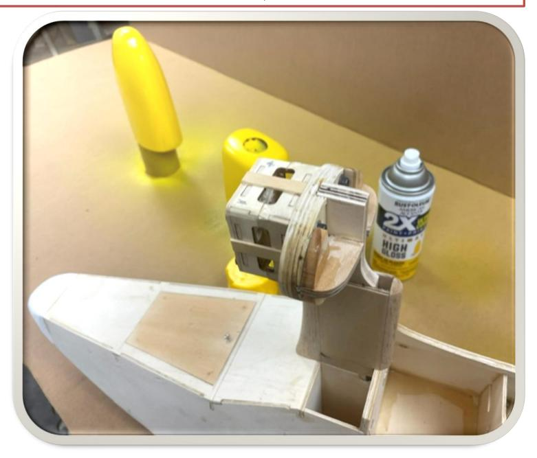
Closeup of motor mount in place!
