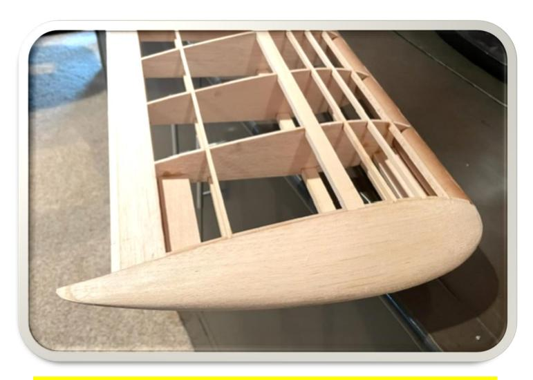
Closeup of the right wing with ribs, spars minus the ailerons!
