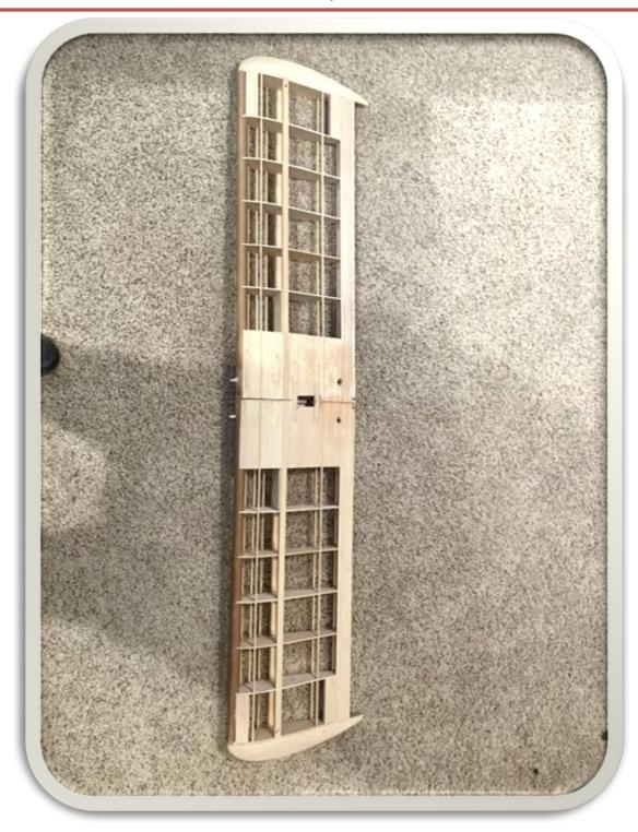
Full wing with ribs, spars still missing the ailerons! Covering needs to be added.
