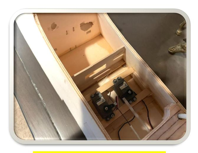
**Closeup of Servo installation in fuselage!**
