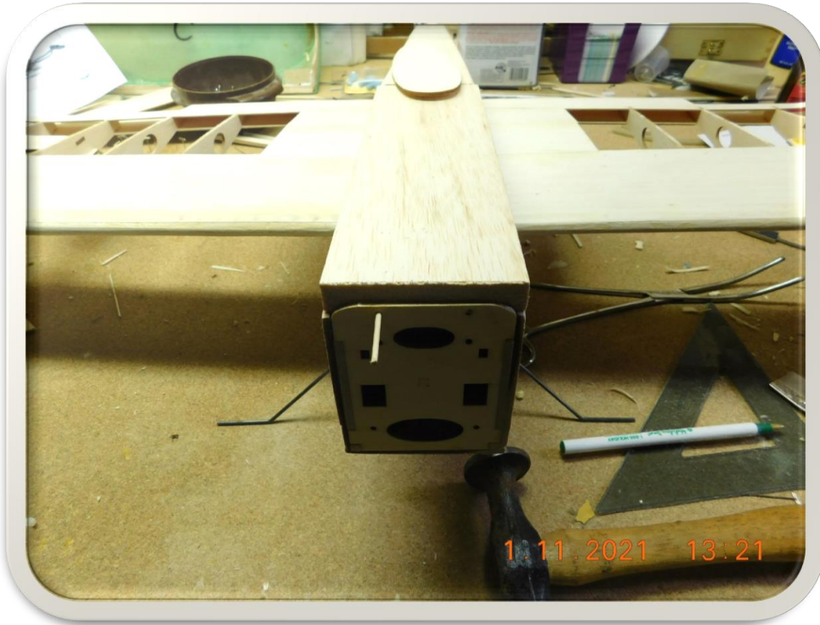
Sheeted bottom of Fuselage and wing center section both top and bottom
