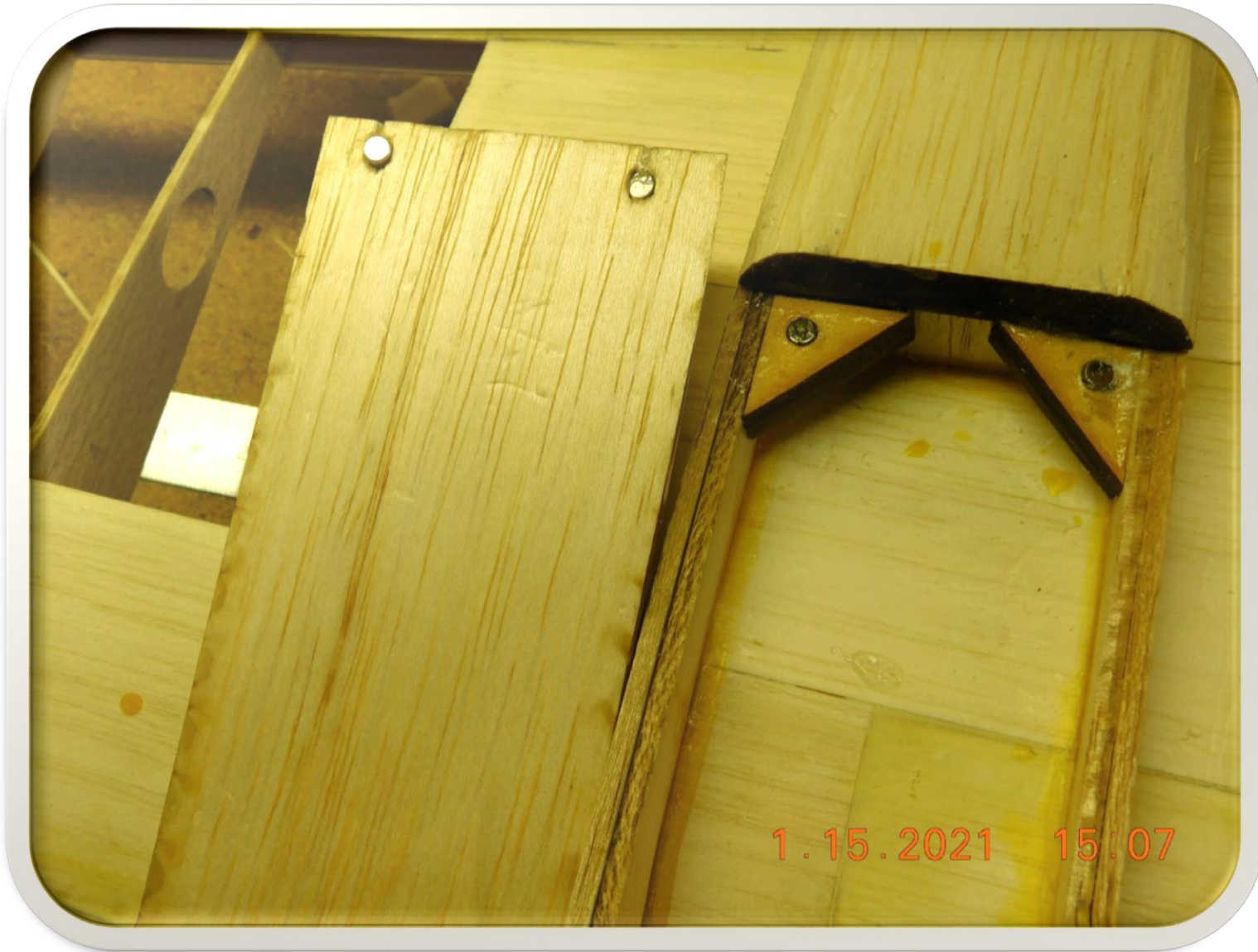
Built the Battery Box Carrier
