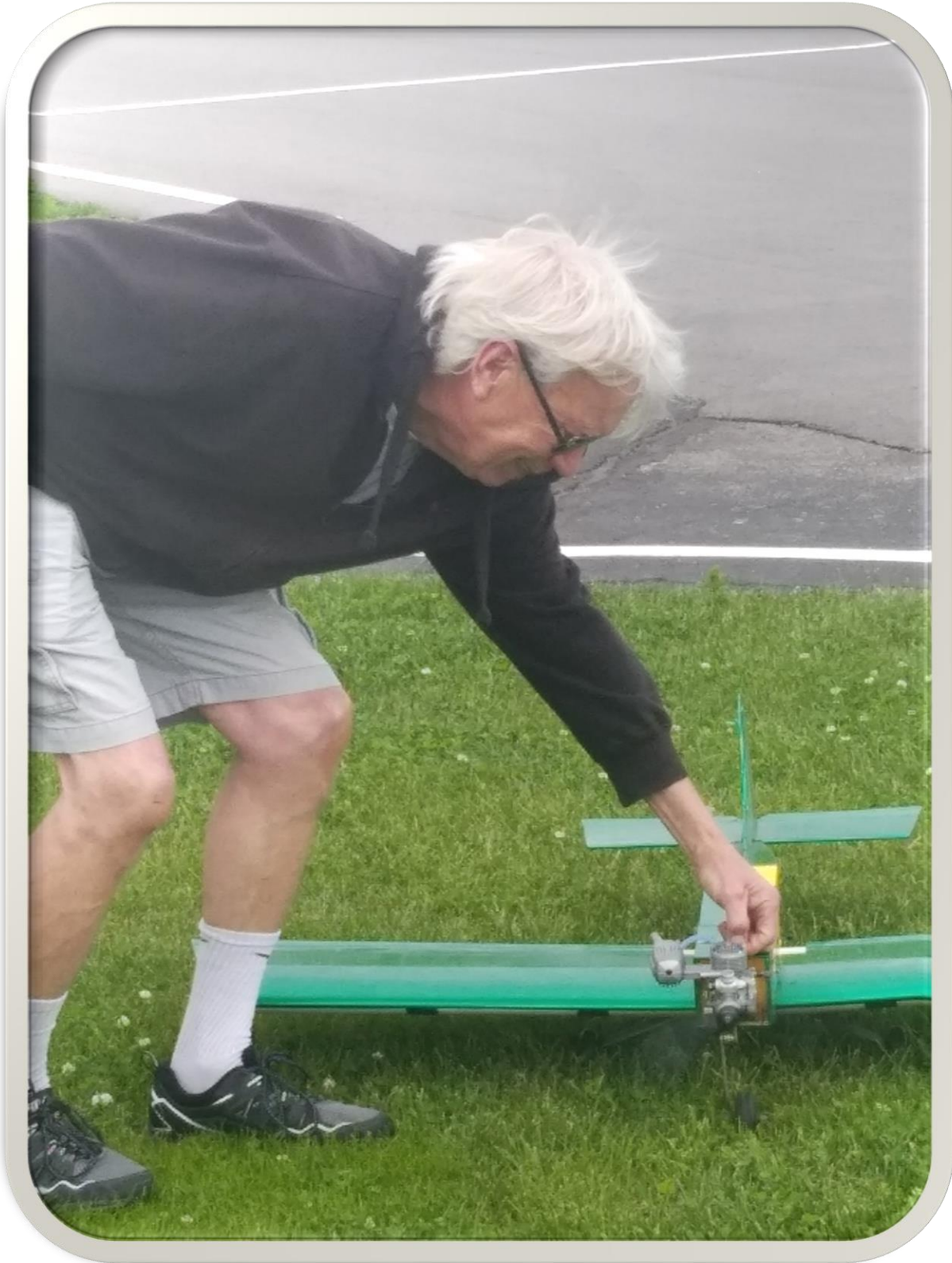
Tim P completing his flight of his father's Midwest Products "Sweet and Low Stick", Motor is OS 46 nitro. Built in the late '80s. you can see him pinching the fuel supply line tight till the engine dies.
