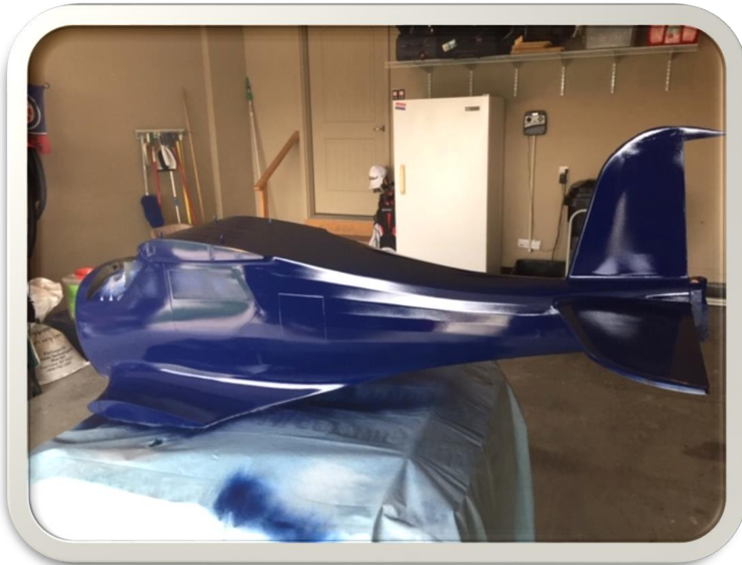
Rustoleum rattle-can paint finish
