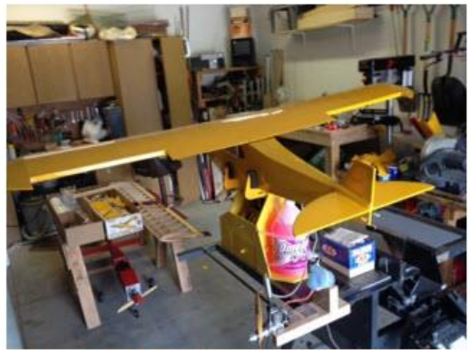
Photo 10- Covered Wing and Fuse
