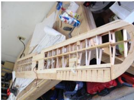
Photo 3 - Completed Wing with Ailerons installed
