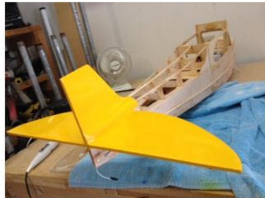
Photo 8 - Covering Fin and Stab
