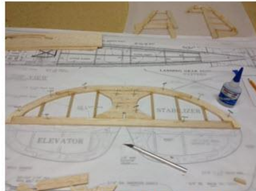
Photo 2 - Showing the Stabilizer Assembly
