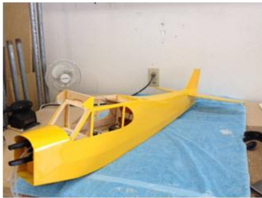
Photo 9 - Covering the Fuselage
