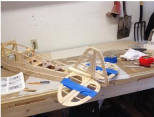
Photo 7 - Installing Elevator and Rudder hinges and pushrods
