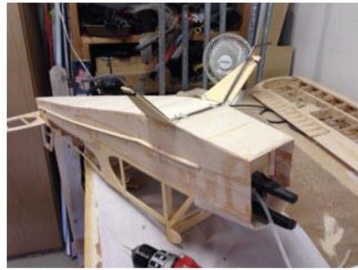
Photo 6 - Installing Landing Gear
