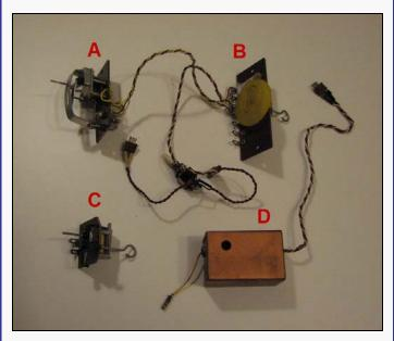
You are looking at a simple escapement, they were used with a single channel radio system and were powered by a rubber band. A signal from the Rx would trigger the coil and allow the rotary part of the escapement to rotate 180 deg. When hooked up properly you would get a linear movement of about 3/4" to operate the throttle.
