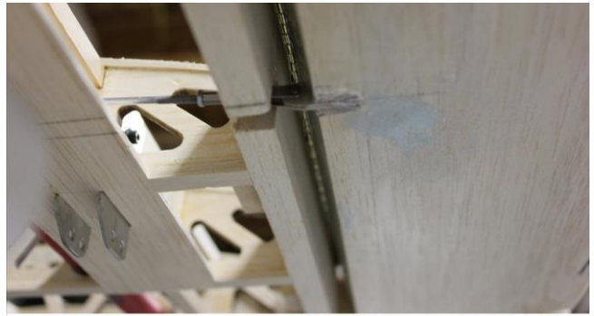
Bottom view of modified aileron linkage and control horn
