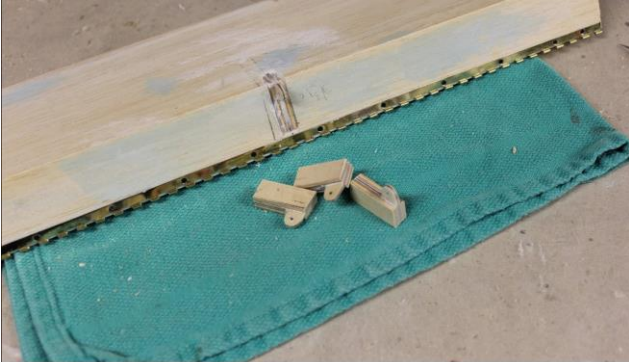
Aileron horns laminated with 1/8 ply Top Left aileron with new horn let into aileron leading edge.
