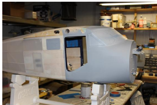
Metal and trim area's defined with high build primer.
