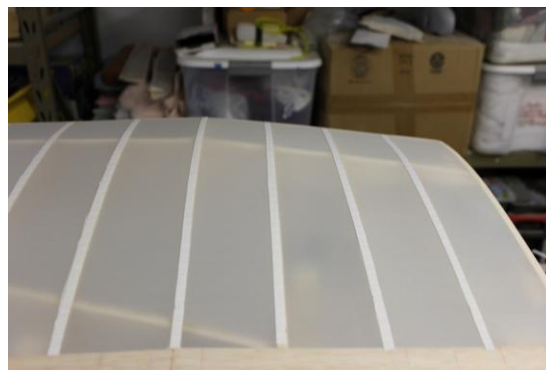
Rib stitch applied to left wing
