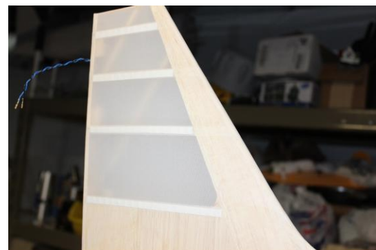
Pink'd (rib) Tape on Vertical Stab
