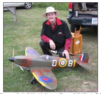
Shown at Springfield with his new Hangar 9 Spitfire is **Neil Kilchriste**. The Spitfire has a 65" wingspan and weighs approximately 8.5 pounds. It takes a .60 two-stroke motor. It is also equipped with retracts.
