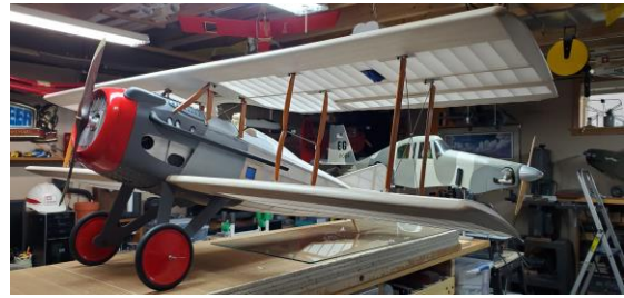
Airframe with two coats of polycrylic.
