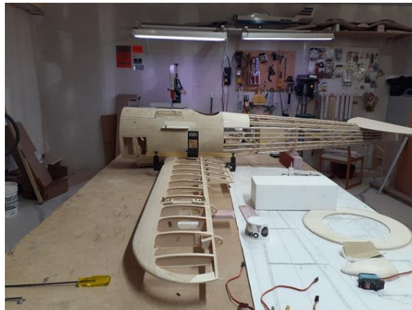
Incidence meter on bottom wing showing +2 degrees. Tail at +3 degrees.
