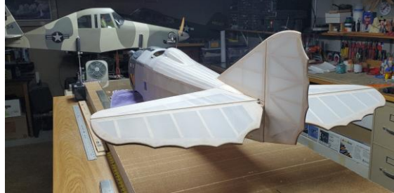
Airframe with two coats of polycrylic.
