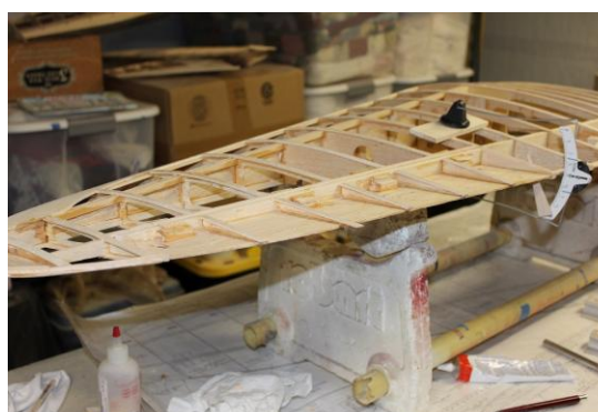
Preliminary check of aileron throw with flat hinges temporarily installed
