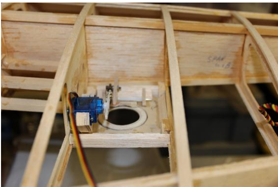
Light assembly in wing retracted position
