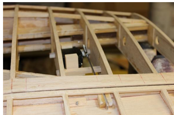
Left wing flap top view servo and horn have been relocated for better linkage geometry
