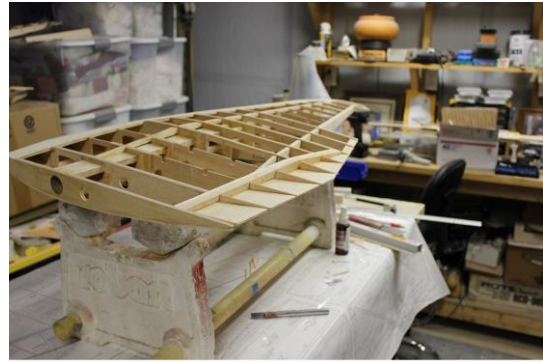
Flap with ribs added left wing bottom view
