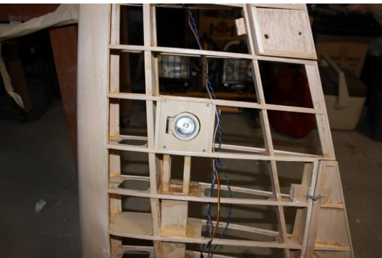
Landing light in retracted position with reflector
