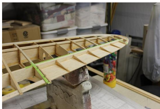
Bottom of left aileron with ribs added
