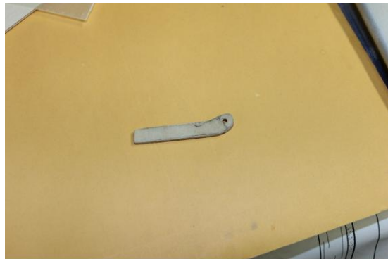
New control horn for flap and aileron made from 1/16 ply and "G-10"
