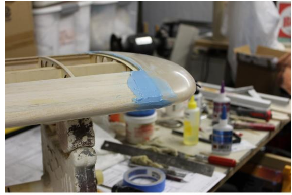
Blending the tips to the wing using super fill
