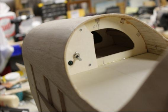
Mockup for master switch
