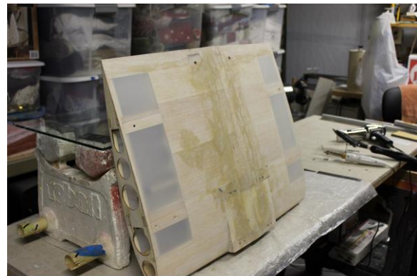
Wing center section in covering
