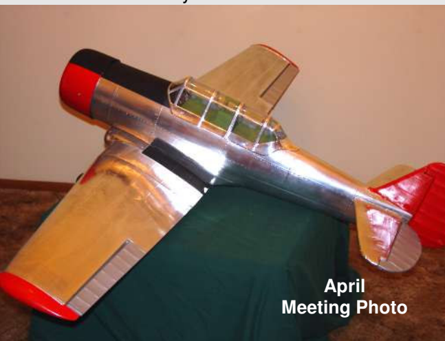
Joe Halamek .015 Aluminum Covered AT-6 Rivets & panels
