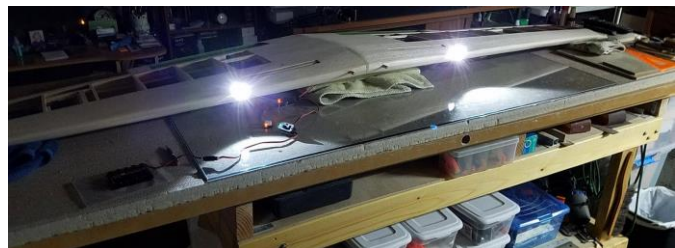
These LEDs put out a strong light. I also use the original reflective bezels from the mini-flashlights to provide more light.
