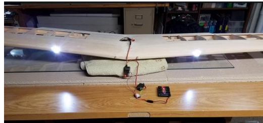
Flap channel turns lights on/off with flap use.
