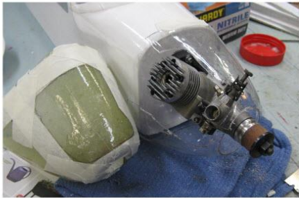
Shrink 2 liter pop bottle over cowl to make a clear sacrificial cowl to be used as an engine cut out guild. Extra step but it doesn't take that long.
