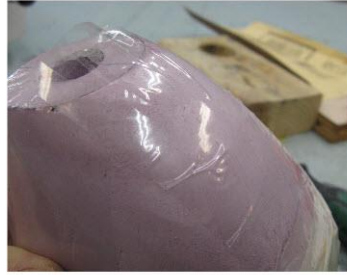
Put clear packing tape on the plug to act as a mold release.
