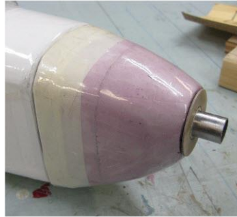
Put clear packing tape on the plug to act as a mold release.
