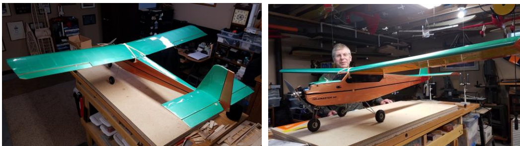
An auction "find" in Kansas City, netted Larry Wosecyna this good looking Telemaster. He has since converted it to electric power. Larry says: "The Telemaster is an older build nicely done, but not on the light side. Power will be provided by an O.S. 5010-810 motor controlled thru a Castle Creations 75 amp ESC. For starters, the prop will be 12x6 and a 4s5000 Lipo pack. This should provide about 750 watts of power for the 7 pound plane."
