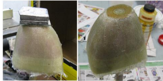
First coat of fiberglass applied. Lead weight used to smooth out the nose of the cowl. Ceramic space heater used to speed the cure time.
