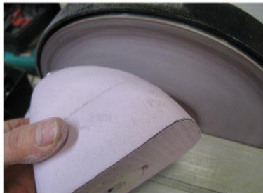
Rough shape of the cowl; notice the fiberglass cowl ring on end of the pipe.
