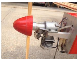
Inverted Super Tigre 56 engine without a muffler before restoration.
