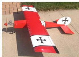
Ugly Stik after restoration. This picture shows the Super Tigre 56 engine mounted upright with a Tatone-Pitts muffler attached
