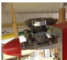
Magnum XL 61 engine replaced the Supre Tiger engine after the first aborted test flight.
