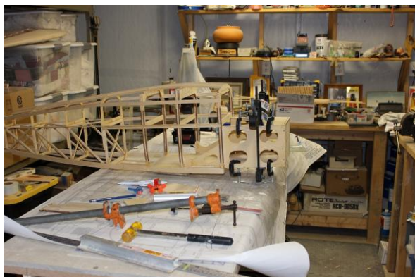
Fuselage with nose formers epoxied in place
