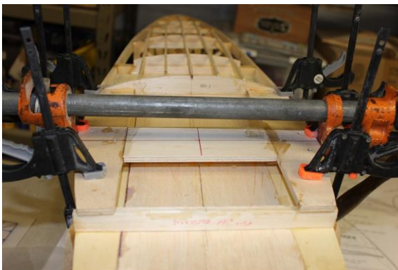
Landing gear rails and cross brace
