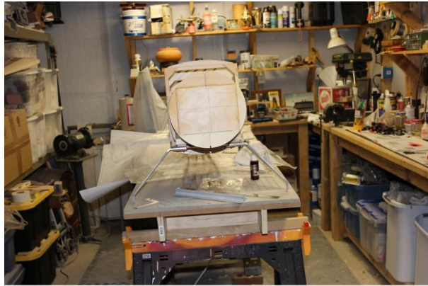
Former parts F-1 glued to nose section
