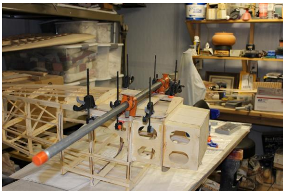
Landing gear rails and cross brace
