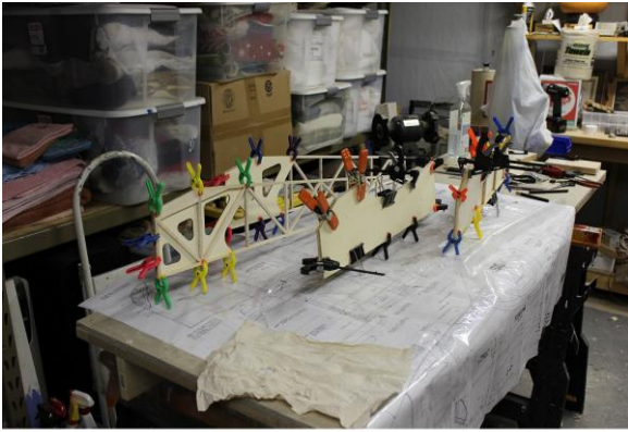
Lite Ply doublers nose and aft section
