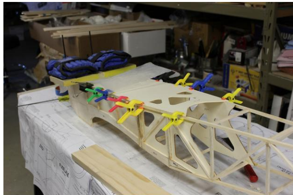
Top doubler joining front and rear sections
