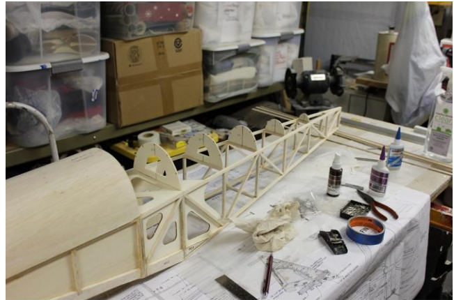
Top formers marked and positioned for stringers
