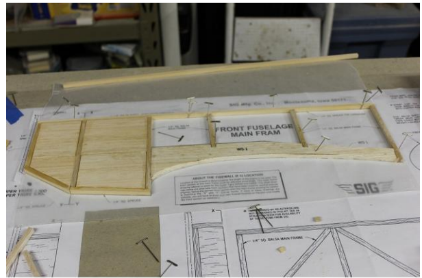
Front half of fuselage with wing saddle, and blocking
