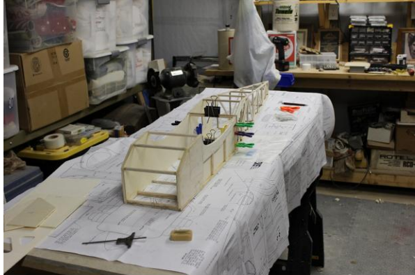
Fuselage sections epoxied together
