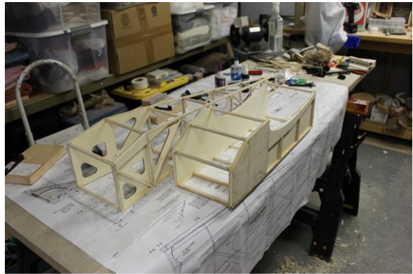
Front and rear sections prior to joining
