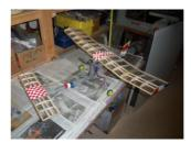
as total weight including battery was 10 ounces. The power system used was a 2206-171 motor, an 18 amp ESC, a 3S 500-800 battery and a 9 X 4.5 prop. It was all
