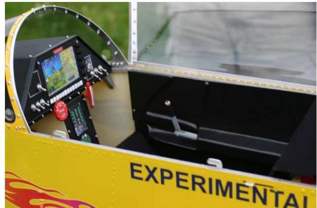
Note the glass cockpit instrumentation. Color radar for approaching storms.
