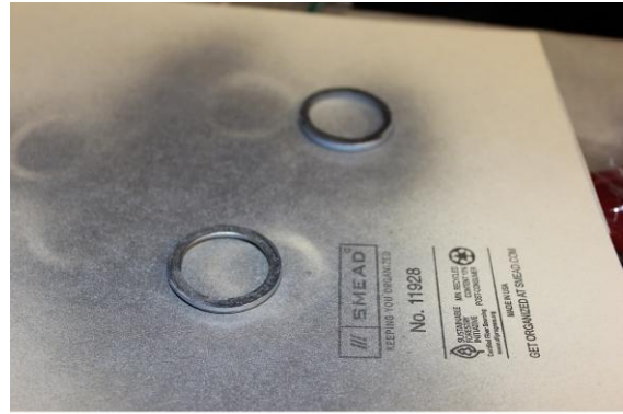
Front of landing lights with paint to bring out the flaws
