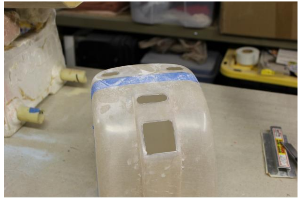
Opening air holes in cowl
