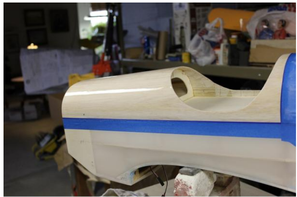
Sealing around cockpit with WBPU, next step primer
