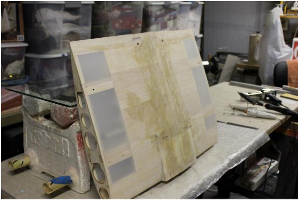
Wing center section in covering
