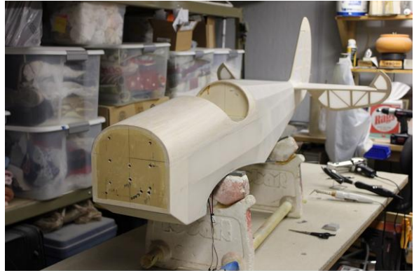
Fuselage covered, ready for finishing tape and primer
