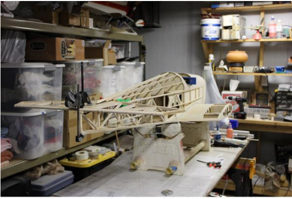
Attaching the stab to fuselage
