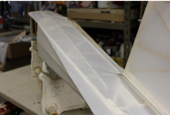
Covering fuselage sides
