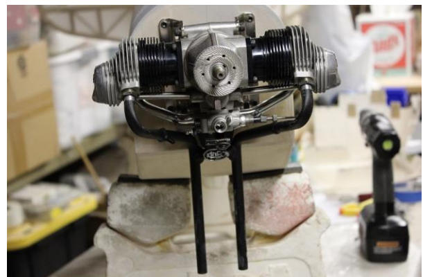
Fitting the new Keleo exhaust
