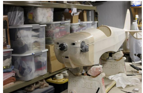
Cowl first test fit
