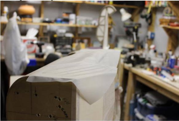
Covering fuselage sides
