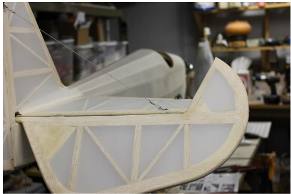
Making up tail brace wires
