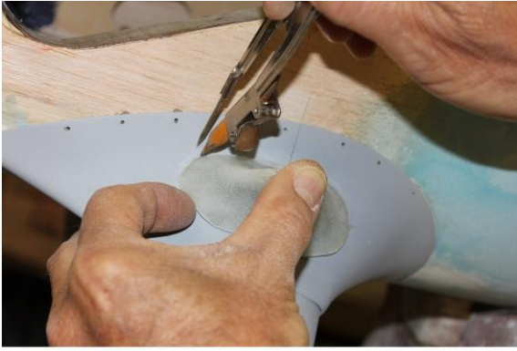
Marking cut lines
