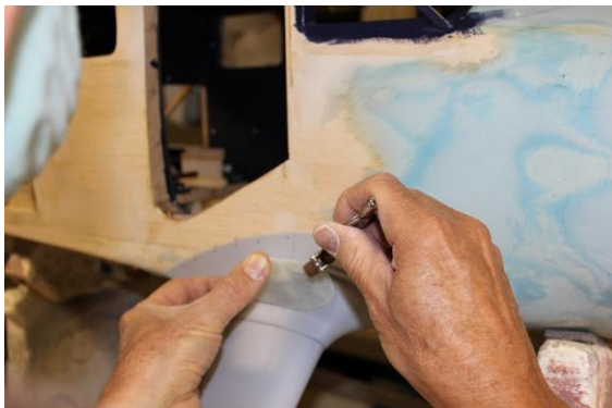
Using compass to mark cut line on strut fairing
