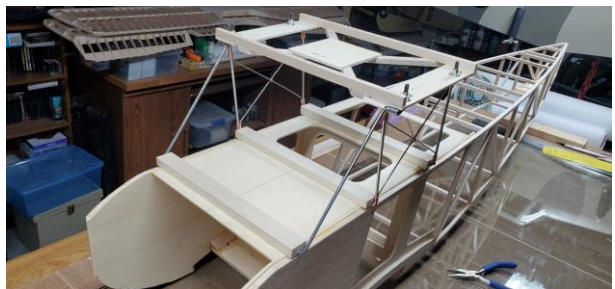
Temporary rigging jig for cabane.
