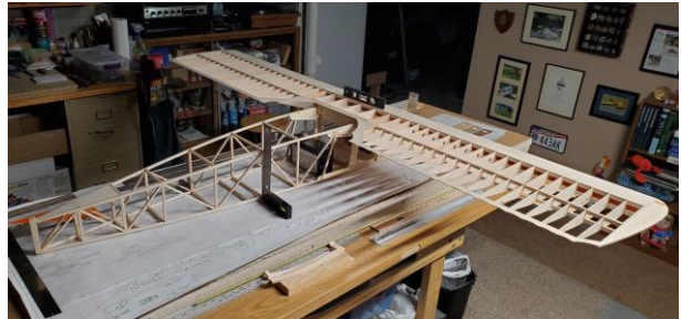
Bottom wing mounted and trued to the fuse.
