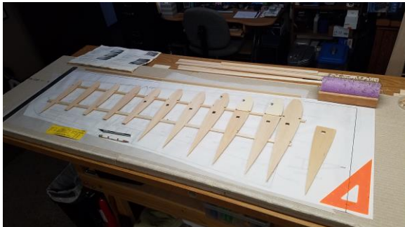
Simple wing construction.
