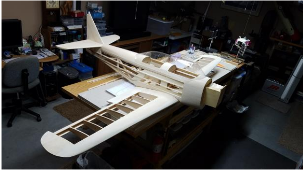
Canopy over tandem cockpits fits well and proportional to scale of airplane. The canopy was meant for an AT-6 kit.
