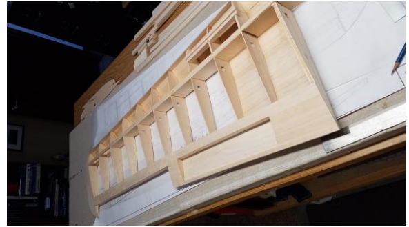
Bottom of right wing showing location that the split flap is retracted. I'll modify the flaps by using a Fowler flap type extension.
