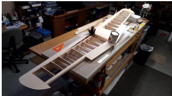
The 89" span wings were set with dihedral less than what called for in the instructions. I raised one wing 7.25 inches, rather than the 9.75 inches.
