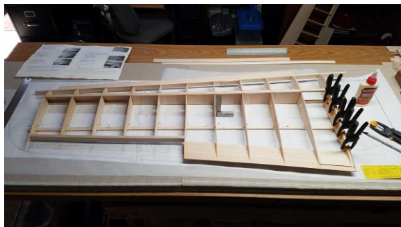
Two servos will be installed in each wing for ailerons and flaps.
