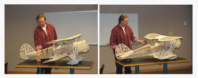
Jim Henley brought a Pica 1/5 scale Waco YMF he has been building for the last several months. With a SISA 30cc gas motor it will weigh approximately 20 pounds. Jim will cover it with Solartex. The aircraft has eight servos, and operating navigational lights including landing lights. Designed into the Waco are several access hatches to access servos, radio, and fuel loading area. Excellent craftsmanship has been exhibited by Jim with this model.
