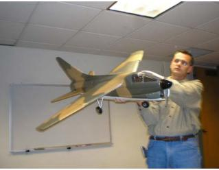
**Jeff Jacobs** brought an outstanding A7 Corsair he scaled up from plans by Rich Urvich. The original plans were for a .20 size glow engine. Jeff has installed an OS Max .70 four stroke in his Corsair. The fighter weighs 7 pounds. You must look closely to see that it is powered by a prop engine. Nice workmanship Jeff!
