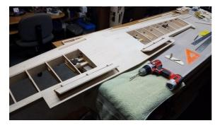
*Du-Bro* pin hinges are used and configured to get the *Fowler* action with the flaps. Servo pushrod enters the wing "pockets" where it attaches to flap leading edge. I should easily get 45 degree flap.
