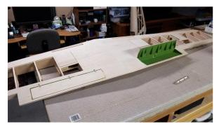
Underside of the flaps and pockets also needed the zinc chromate green coating.
