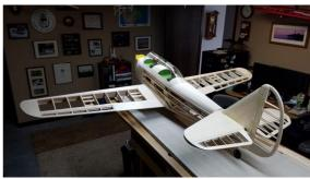
All the components have been built. These three photos show a mock-up of the PT. The VVRC 20cc gas engine is already fitted to the firewall. Just need to mount and plumb the fuel tank. *Ultracote* will be used to cover the model.
