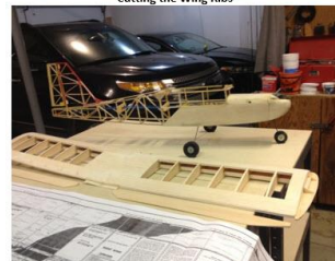
Joined Wing Halves with Sheeting
