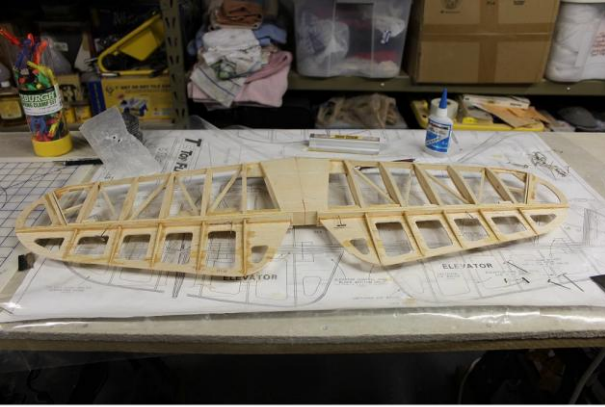
Stabilizer and elevators
