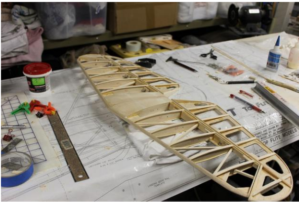
Stabilizer and elevator frame out complete
