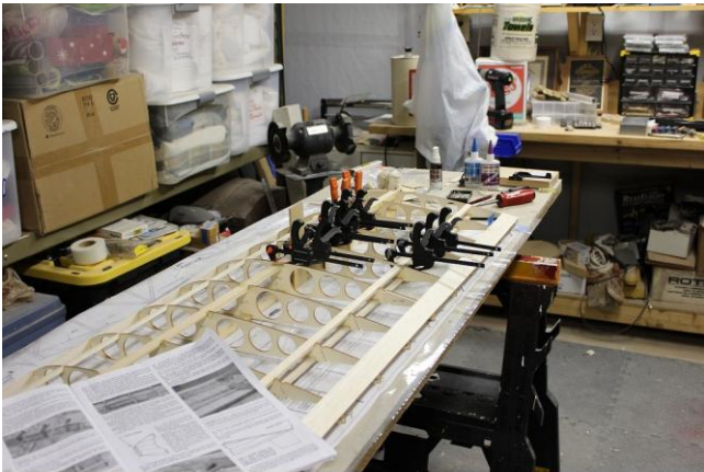
Wing joiner / mount/shear web assy, epoxied between the upper and lower spars
