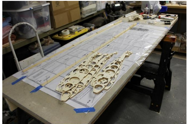
Laminated wing spars, rib sub assemblies.
