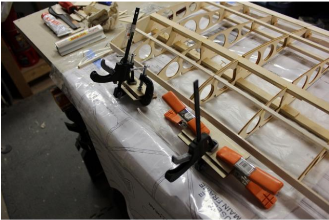
Another view of the wing joiner mounts and shear web assy.
