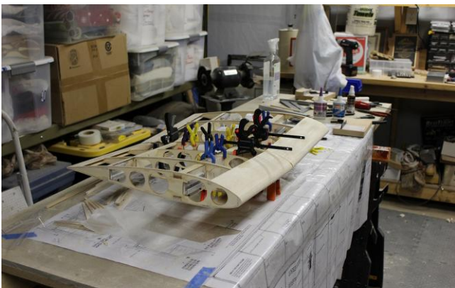
Wing center section, epoxied together
