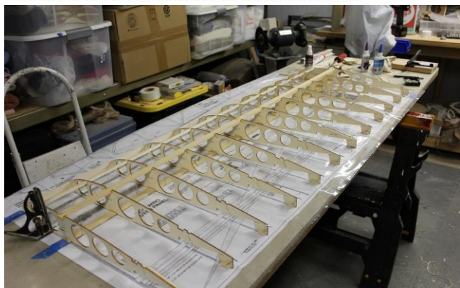
Wing frame with leading edge, upper and lower spars
