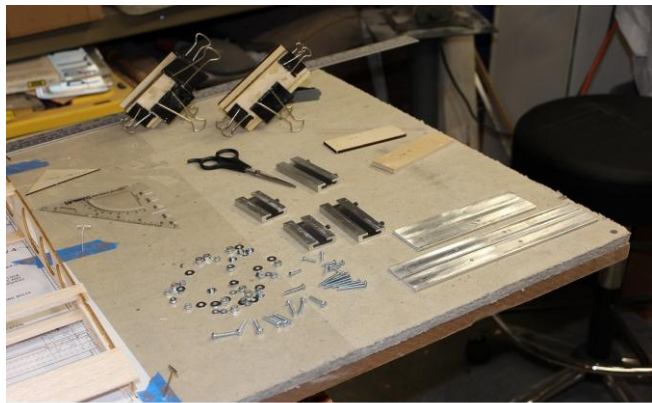
Close up of wing joiner hardware and plywood shear web sub assemblies
