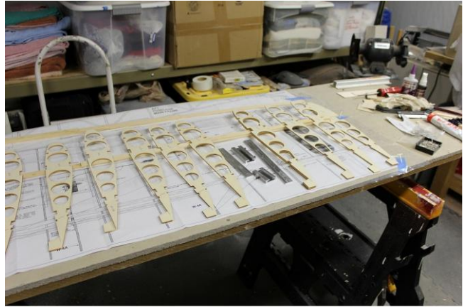
Wing Joiner hardware, ribs laid out according to the plan
