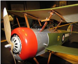
Material choices: I made most of this airframe from Depron, some wood sub-structure, spars, and ribs to hold shape. Wood was balsa and bass. Airfoil was 'baked' in the oven, most contours were pre-formed by rolling. Rib tape, and small details were 20lb. bond paper to 100lb. index card stock.
