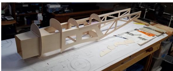
Fuse plan with "greenhouse" canopy propped over the sheet.
