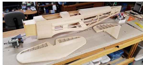
Open cockpits of sheeted fuselage and sheeted horizontal and vertical stabs. The two cockpit openings are larger than the "two-holer" PT-19.
