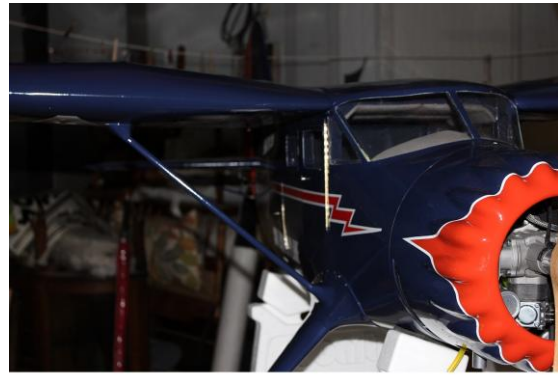
Wing strut Landing gear fairing
