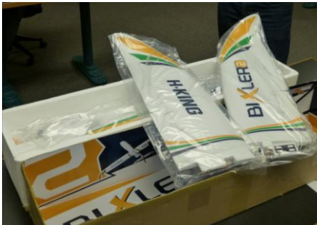
The Bixler II is a foam ARF with a 59.5" wingspan. Electric motor is rear facing and Tim will use 2200 mAh battery packs.
