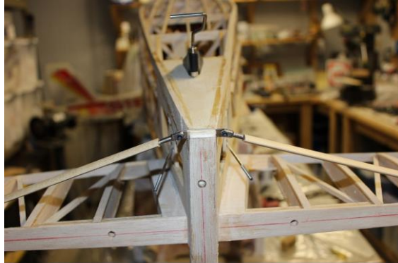
Tailbrace mounted to fuselage
