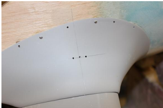
Landing gear fairing, marking opening for wing strut
