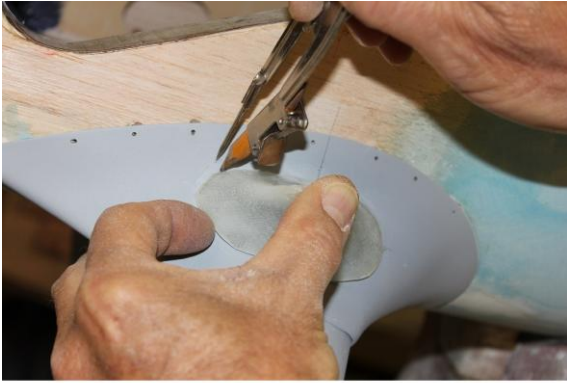
Marking cut lines
