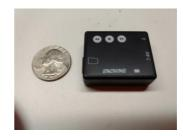
However, I'm still plugging away. I recently purchased a DVR (digital video recorder) that I can plug into my fpv goggles and record the flight video. It is an Eachine EV1000 DVR, a rectangular box 1.5" x 1.25" by .5". It uses a memory card similar to those used by digital cameras. I have a 32 GB card for mine and it does a decent job of recording. If you are interested, here is a link for a recent YouTube video https://youtu.be/YGqZDuBmI7A
