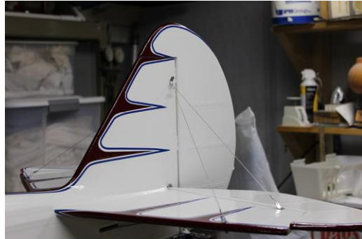
Tail Brace Wires
