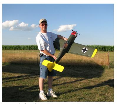
Member <u>Rick Johnson</u> with his M.E. 109 built from a Wing Mfg short kit. It has mechanical retracts and powered by an O.S. Max FP .40. Rick has been flying for over 10 years, and handles his 109 well off the grass field and over the tall corn.
