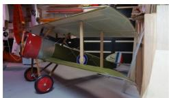
NOTE: Wingspan is 108", engine is a Zenoah G62 swinging a 27" X 6" prop. Ready to fly weight will be between 32 and 33 lbs.
