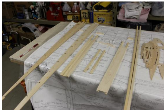
Wing sub assemblies, Main spar spar web, trailing edge spar, inner t.e. spar
