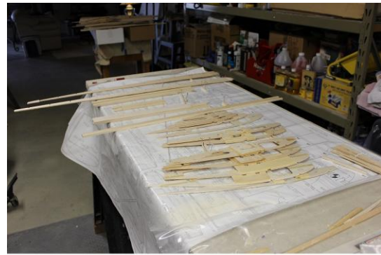
Wing sub-assemblies (ribs)
