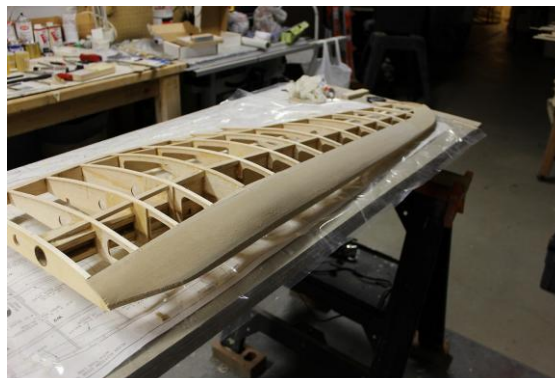
Left wing with sheeting and cap strips from root end
