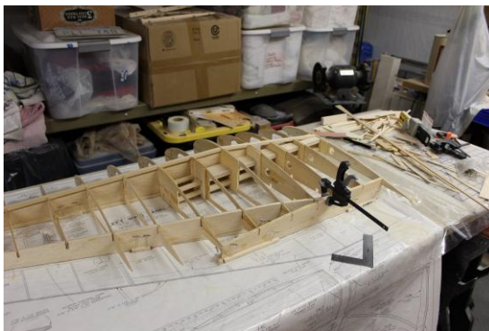
Wing frame up no glue applied yet
