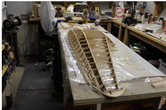
Basswood leading edge spar from wing tip
