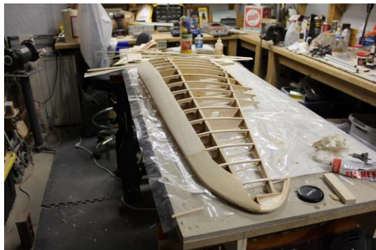
Left wing from tip end, all sheeting and cap strips applied
