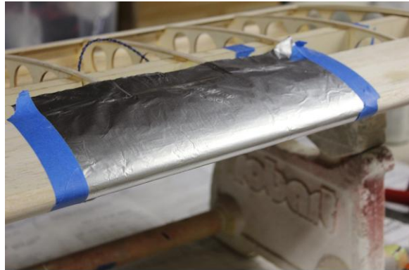
Non stick aluminum foil. Landing light cover will be moulded over this
