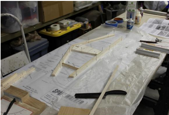
Start of horizontal stabilizer framing
