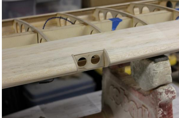
Test fit light bracket in wing leading edge
