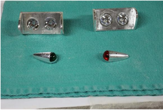
Finished navigation lights and landing lights
