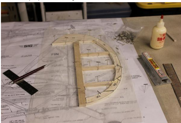
Rudder framed up
