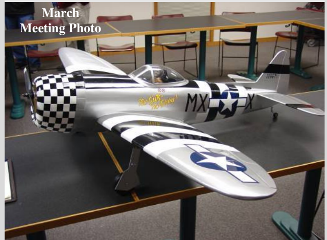
Joe Halamek's new Hanger-9, P-47 Jug ARF - Magnum .91, retracts, This aircraft builds Very Light .
