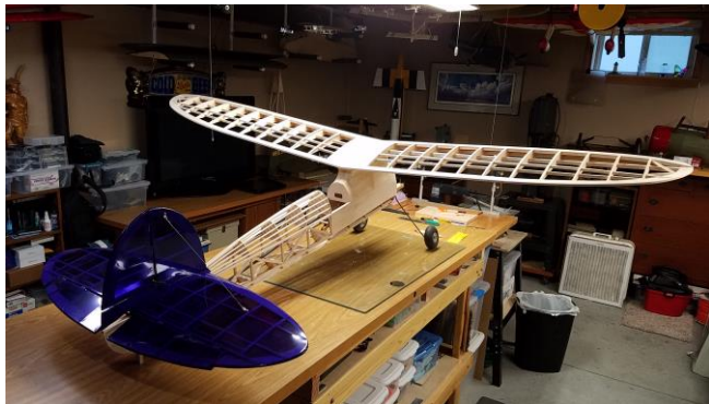
Gear installed and purposely angled forward with use of heavy wheels to get the CG forward more.
