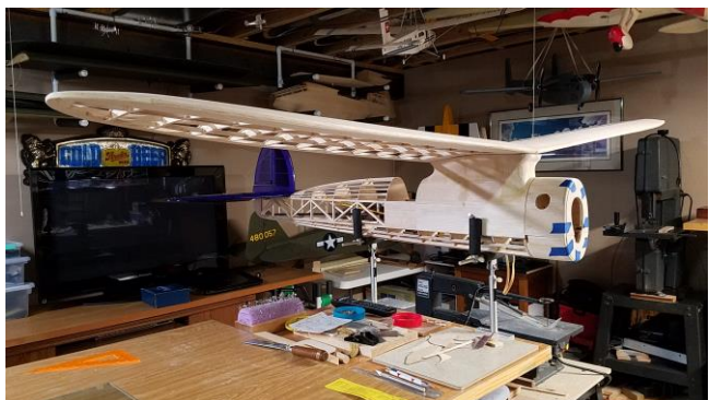
Nearing completion. Balsa sheeting to be fibreglassed along with the cowling.
