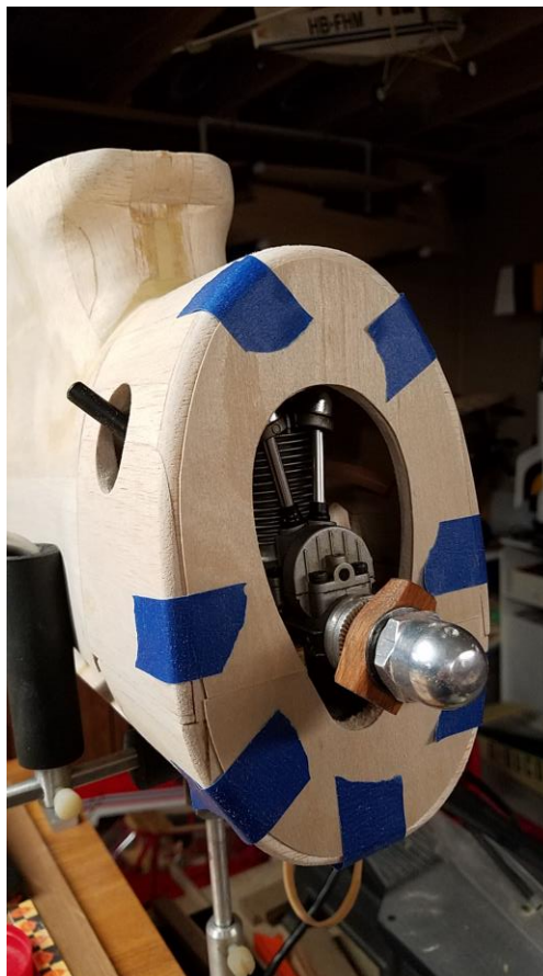
Saito .45 exposed in "keyhole" with exhaust pipe extending out the side.
