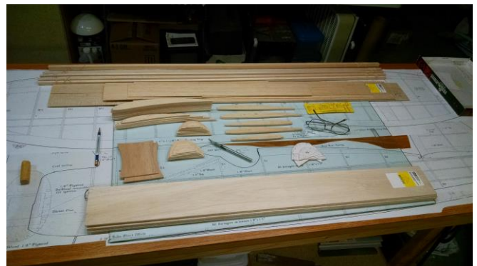
With an extra plan sheet, I made templates for the ribs and turtle deck bulkheads.
