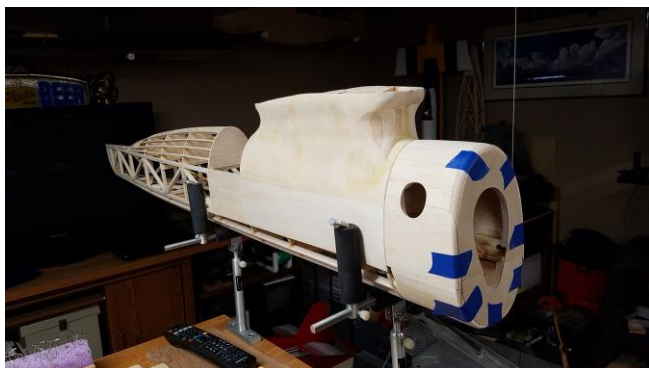
Top 2/3s of cowl removable. Large "exhaust" port for either pipe or muffler clearance.
