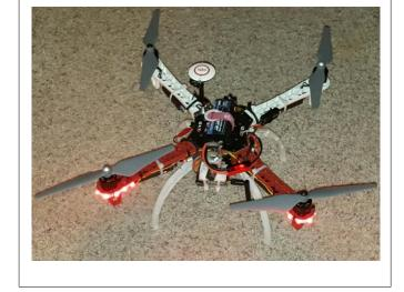
Here is the top of the quad copter. It uses common 3s batteries
