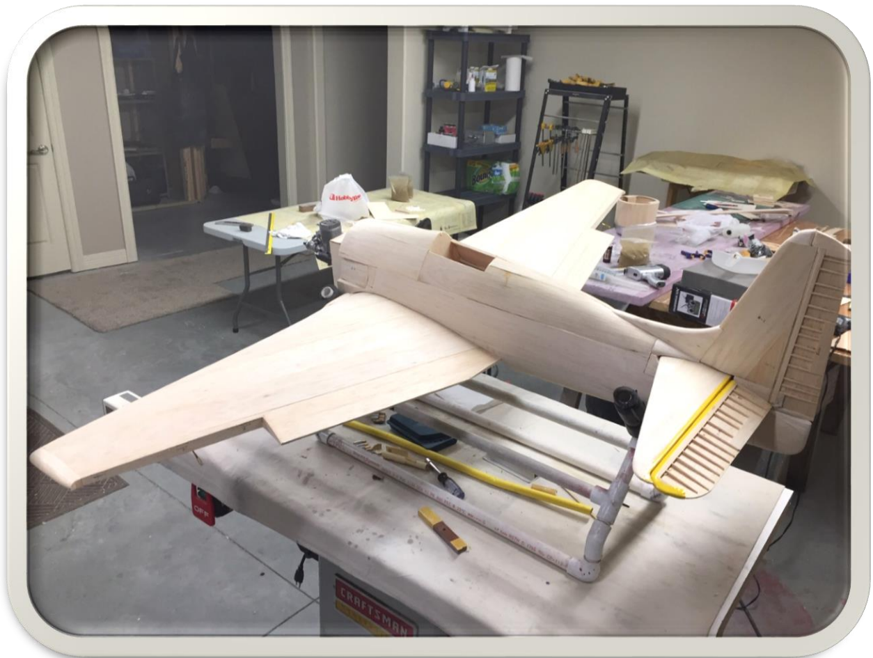
Bernie mods the wingspan of the tapered wing at the root
