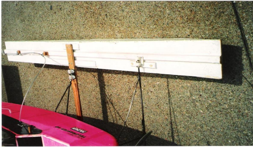
One way to spread and fasten the floats. Setup has diagonal bracing on rear landing gear, laminated hardwood connecting the rear floats and one water rudder.
