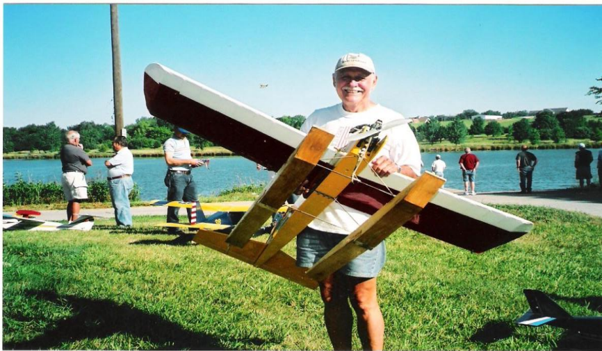
Much used LT 40 with OS 52 FS and Cunningham floats. Floats have thin ply on bottom. Setup has no diagonal bracing, normal landing gear spread & one water rudder. Pilot-Bob Zitzsperger.
