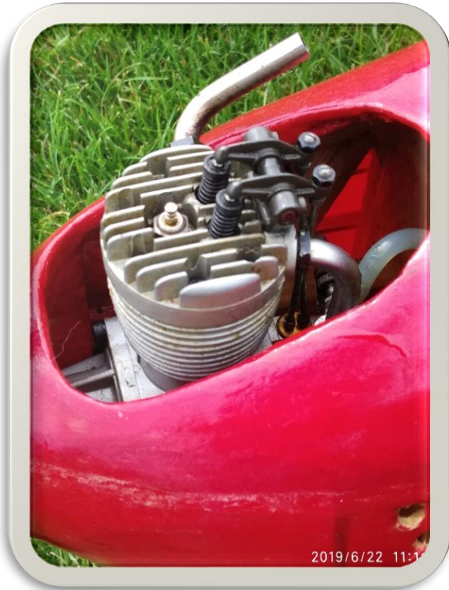
Close up of Bud's 4 stroke with open rockers (Photo by Joe H)
